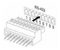
\* When RS-422 connection is being used, do not use RS-232C connection.
