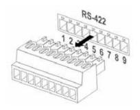
2. Peel off a section of copper wire (AWG Nos. 28 to 18) and insert it into the connector hole; then use a flat head screw driver to fix it
