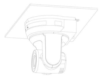
3. Remove the screws on the hanger and the machine
