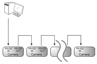
With RS-232 in/out, at most 7 CVs can be connected.
