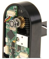
The tilt clutch adjuster is accessed by removing the Main Cover. This has 3 screws. Take care not to damage the sealing gasket. The Tilt Shaft Support Bearing may be on the shaft, as in this picture, or may me retained in the main cover. Take care not to lose this bearing.
