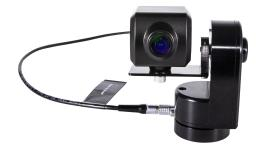
The **CV-PT-HEAD** ( $\mu$ L) can be controlled by CV-MICRO-JYSTK or any BR Remote style controller. These controllers generate RS485 data which can be connected directly to the CV-PT-HEAD or sent via an IP network with IP adaptors. The RS485 data can be sent up to 3,000+ feet (1km) on a four (4) pin XLR cable.
