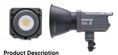
The amaran 100x S is a 100W bi-color Bowens Mount point-source light with integrated controls, versatile power options, and an upgraded LED chipset for increased color quality and spectral reproduction.
